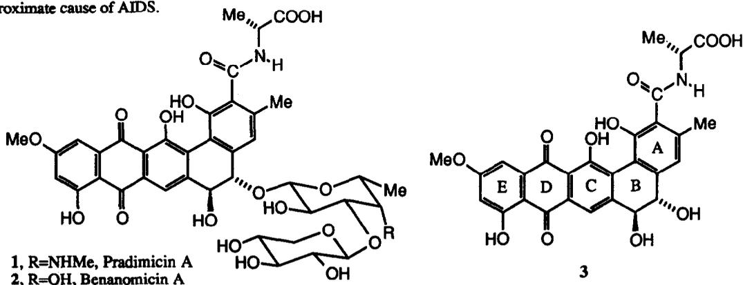
As one component of a program directed toward the development of an efficient and general synthetic route to 1, 2, and analogs thereof, we required a means of constructing the aglycone 3. To our mind, the principal challenge presented by 3 involves the introduction of the two chiral centers of the B ring, but no method known to us offered a simple solution that addressed both the relative *and* absolute stereochemistry of those two chiral centers.
